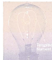
Filament provides resistance to the flow of electrons.
